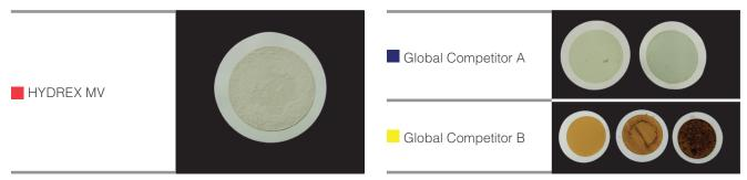
Filters were changed when filter plugging inhibited fluid flow. HYDREX MV's filter only required one filter over the test duration.
